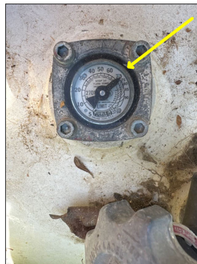
The gas gauge at the propane tank indicated that the tank had 70 % remaining.
